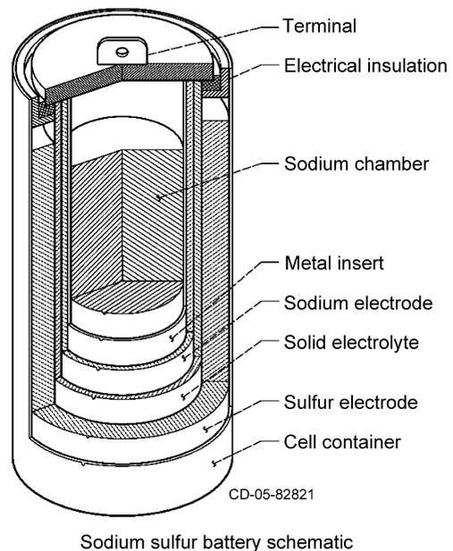
Sodium sulfur battery schematic
