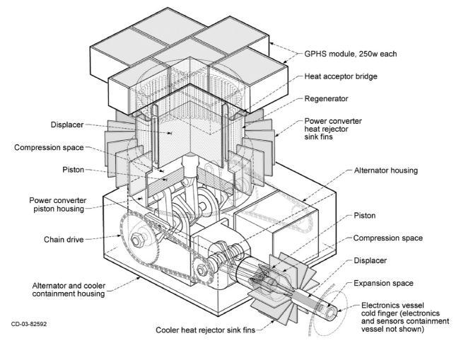
Fig. 2. Power converter and cooler.
