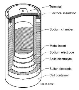
Sodium sulfur battery schematic
