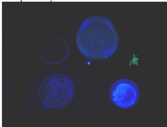
Figure 3. Same samples as figure 1, seen with a standard digital camera (Casio EX-RZ10) in darkness, with samples illuminated with a near-UV LED flashlight (390nm). The sand is totally dark ; some faint fluorescence is seen from the quinine solution and the phenanthrene, and strong yellow fluorescence from coronene.
