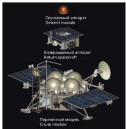
Three elements of the Russian Phobos sample return mission are the cruise stage/lander at bottom, Earth return spacecraft in the middle and the sample return capsule that will ride the Earth return spacecraft back, then dive into Earth's atmosphere. Launch is set for 2009 for a three-year round-trip and Earth landing in 2012. Credit: LAVOCHKIN PHOTOS
