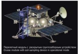
Integrated spacecraft is shown as it will appear on the surface of Phobos, with blue drilling rig mounted on the side. The device can swivel to find the best sample location.
